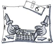
Remove the briquette from the press
